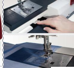
The MC9900's needle plate has numerous guide lines, including angled lines to help you position your fabric exactly 1/4" from the cut edges, perfect for piecing and inset seams.
